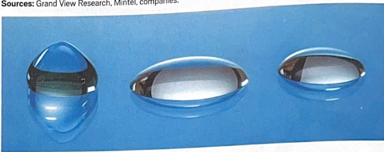
Longer-chain, higher-molecular-weight hyaluronic acid forms stiffer, more viscous water gels. Shown here are water gels with average weights of 2,000, 1,000, and 500 kDa (left to right).
