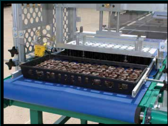
Expanded plug on dibble unit
